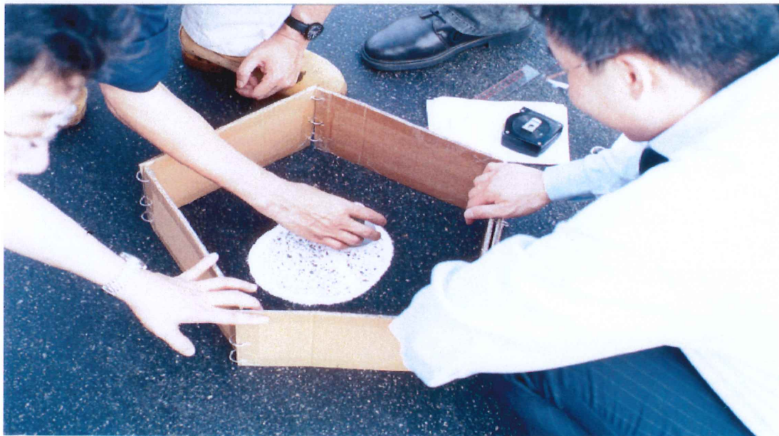
Figure 4.5 Water Penetration & Sand Patch Test
