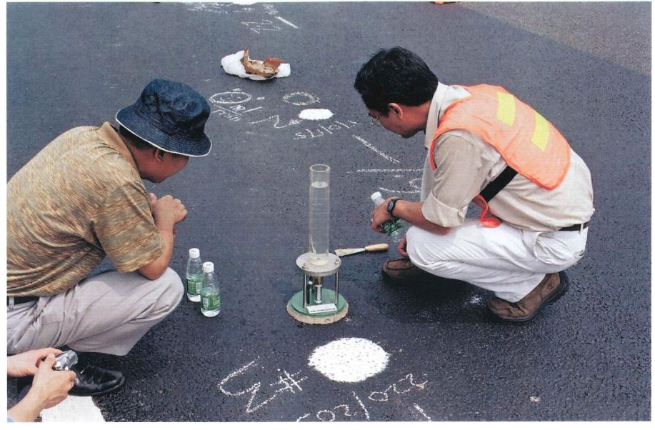
Figure 4.4 Water Penetration Meter
