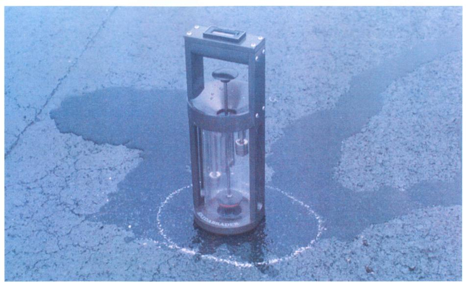
Figure 4.5 Humble Equipment Co. Outflow Meter
