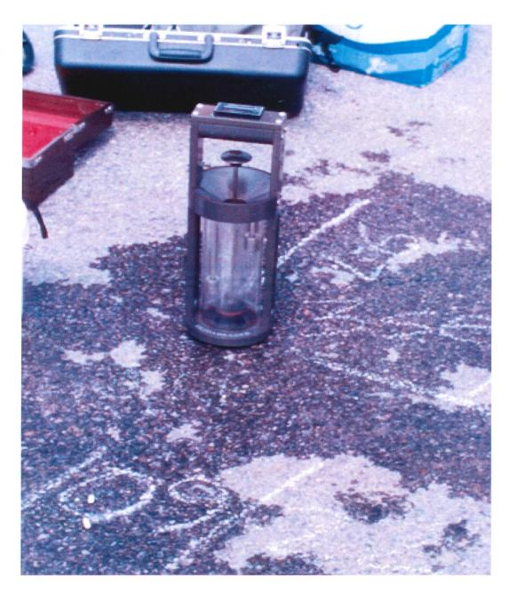
Figure 4.5 Outflow Meter Test
