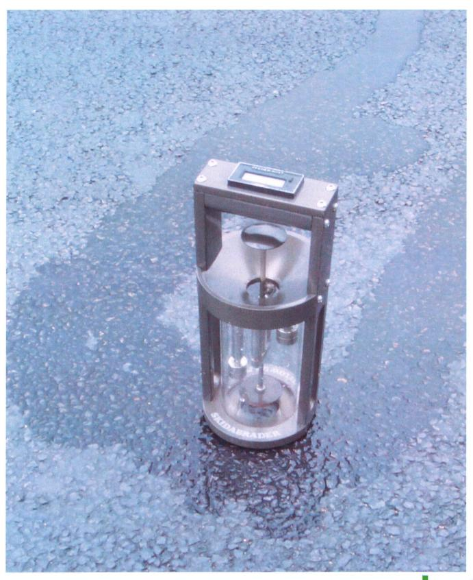
Figure 4.6 Humble Equipment Co. Outflow Meter
