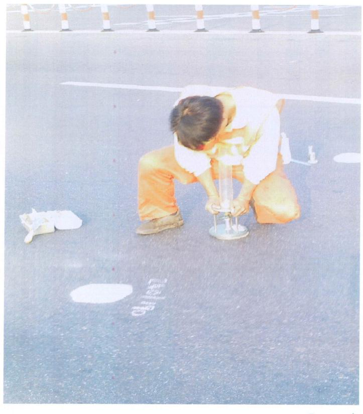
Figure 4.6 Water Penetration Test
