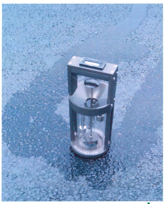
Figure 4.6 Humble Equipment Co. Outflow Meter
