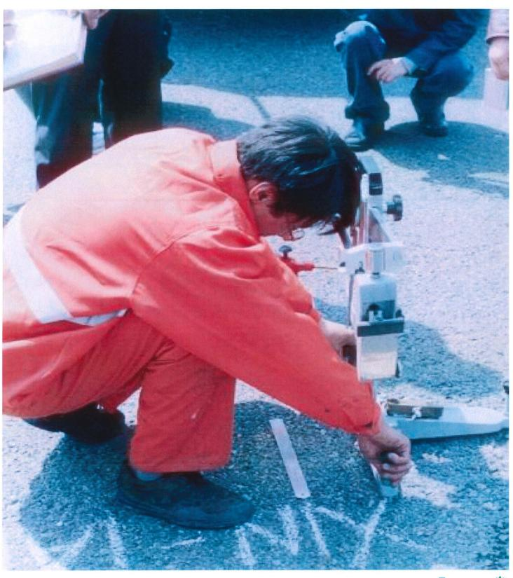
Figure 4.7 British Pendulum Test
