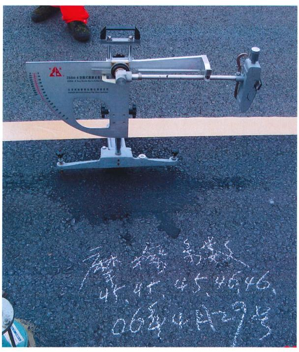
Figure 4.6 British Pendulum Test
