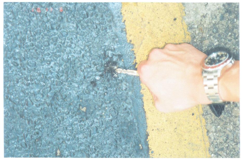
Figure 4.4: Test hole to show depth of penetration of RejuvaSeal <sup>™</sup>
