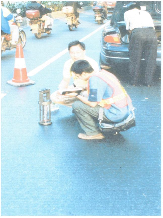
Figure 4.5: Humble Equipment Co. "Outflow Meter".
