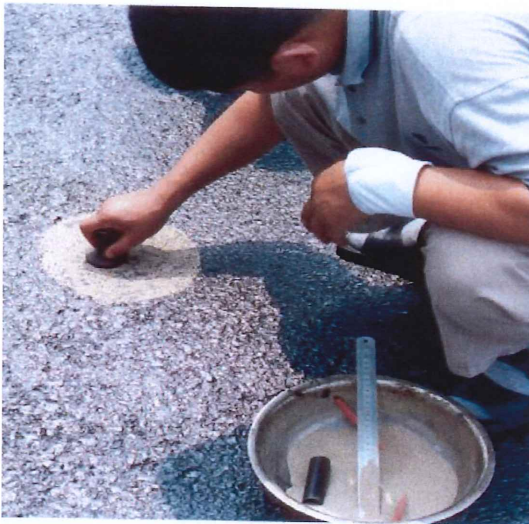
Figure 4.4 British pendulum Test (top) Sand Patch Test (lower left) Water Infusion Test (lower right)
