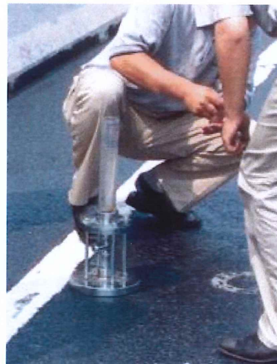
Figure 4.4 British pendulum Test (top) Sand Patch Test (lower left) Water Infusion Test (lower right)
